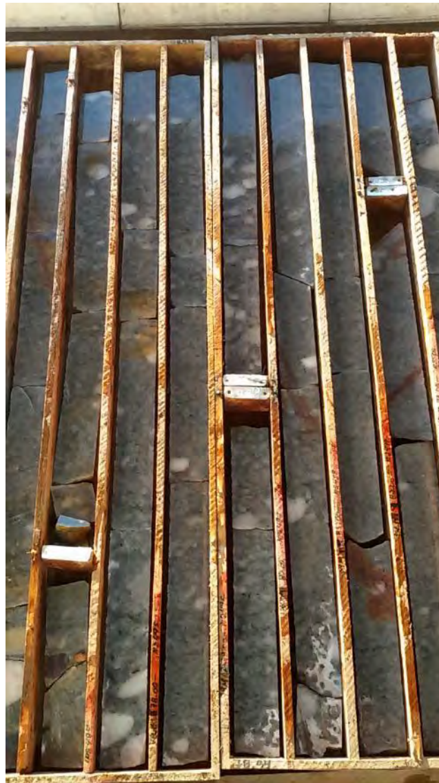
Figure 16-7 Drillcore boxes showing fresh rock zone with one fracturing family with high RQD values and high fracturing spacing
