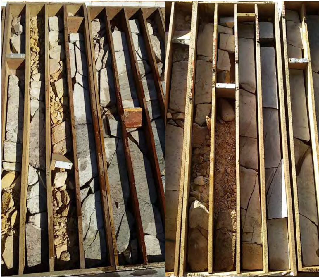
Figure 16-5 Drillcore box in transition from saprolitic to fresh-rock zone with local friable intercepts (shallow than 43m depth).
